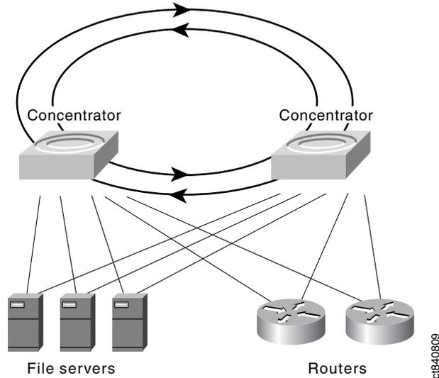
One pair of concentrator links is declared the active link; the other pair is declared passive. The passive link stays in backup mode until the primary link (or the concentrator to which it is attached) is determined to have failed. When this occurs, the passive link automatically activates.
